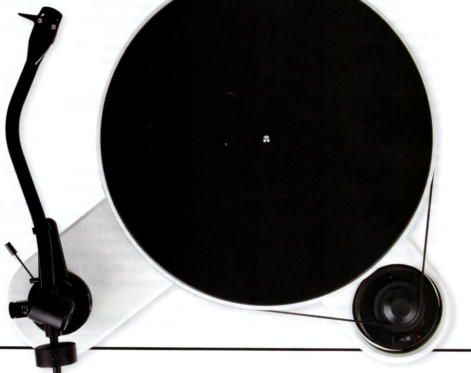
RIGHT: The motor sits in a dedicated hole in the plinth, offering manual speed change for 33 and 45rpm via a stepped pulley. Vinyl topped MDF platter is dynamically balanced at the factory
